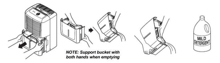
NOTE: When the bucket is full or removed from the machine, the compressor will turn off, but the fan will continue to run for a few minutes. This is completely normal. The dehumidifier will not be removing moisture from the air at this time.
